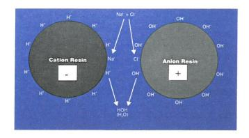
Ion exchange is a chemical process by which ions, or ionic substances that are considered undesireable in water, are decreased or are removed from the water by use of properly designed ion exchangers, or resin.
