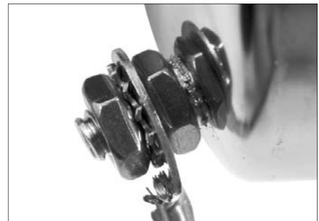
Step 16 - Install Nut on Stud against Washer & Tighten with 7/16" Wrench
