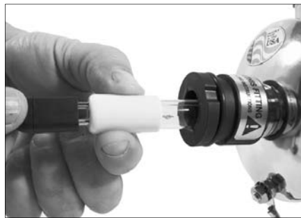
Step 3 - Remove Socket
