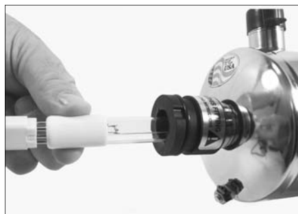
Step 3 - Remove Socket
