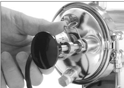
Step 1 - Lift wiper clip up
