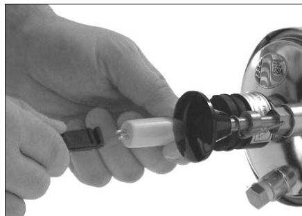
Step 4 & 5 - Remove Sockets
