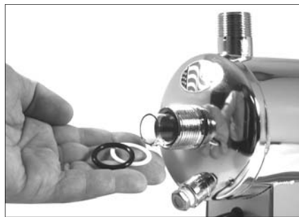
Step 5 - Remove Washer & O-Ring
